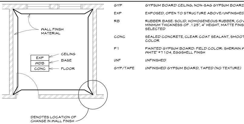
GYPSUM BOARD CEILING; NON-SAG GYPSUM BOARD EXPOSED, OPEN TO STRUCTURE ABOVE/UNFINISHED RUBBER BASE: SOLID, HOMOGENEOUS RUBBER, COVE BASE WITH TOE, MINIMUM THICKNESS OF . 1 25", 4" HEIGHT, MATTE FINISH, COLOR TO BE SELECTED
